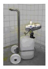
The 672 Drum Mount includes a one-turn control valve to allow you to adjust liquid output (0-300 ml/min) and droplet size (intermediate fog to heavy wet fog). Higher flows produce larger droplets.
