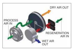
The Silica Gel wheel is continually, slowly rotating, typically at three revolutions per hour. As the wheel rotates a small portion passes through the regeneration segment. During this phase a second air stream (Regeneration Air) is heated to a high temperature before passing over the wheel. Any moisture present in the wheel is released into this air stream, this hot wet air is then exhausted outside the area being dried.
